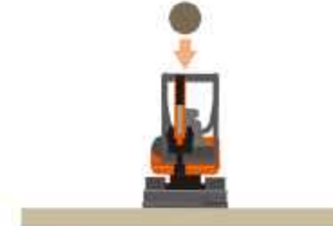
FOPS Falling Object Protective Structure
