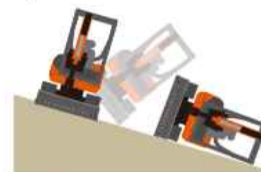
TOPS Tip Over Protective Structure
